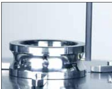
The world-leading gauge delivers 4 mm of range, twice the range of most roundness instruments. This enables the unique capability of roundness, contour, and roughness measurement from a single gauge.
