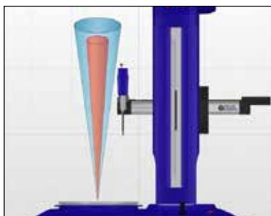
The smaller the coning error of any instrument the more reliable the results. In fact, coning error is the single biggest source of error when measuring cylindricity, parallelism and roundness of tall components.
