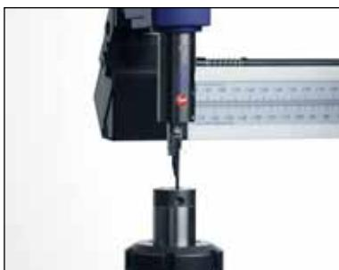
Taylor Hobson's patented method of gauge automatic attitude/orientation\* combined with the "any attitude" Talymin 6 gauge ensure easy access the most complex of components.
