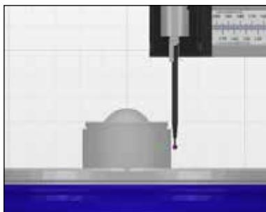
A simple approach to gauge calibration that literally takes seconds to do. Utilising the instrument high precision scales this procedure calibrates both the gauge gain and crutch angle position in a single user guided operation.
